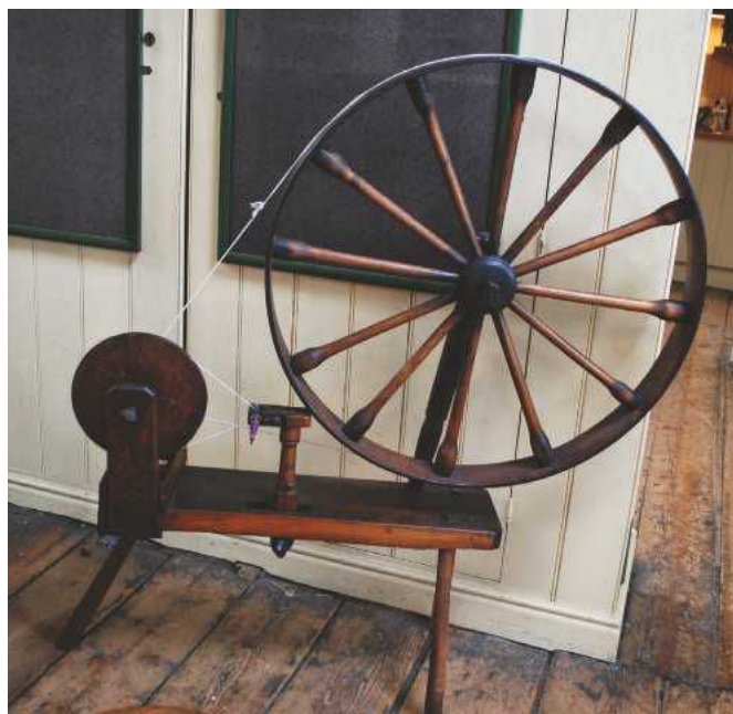
PIRN winder which looks like a spinning wheel. This machine wound the silk onto the shuttle bobbins (weft). Originally wound by a handle, mostly by children, later the machine was run by electricity.
