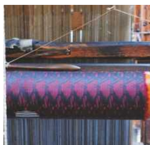
Woven silk using the Jacquard loom. Notice the shuttle on top of the silk
